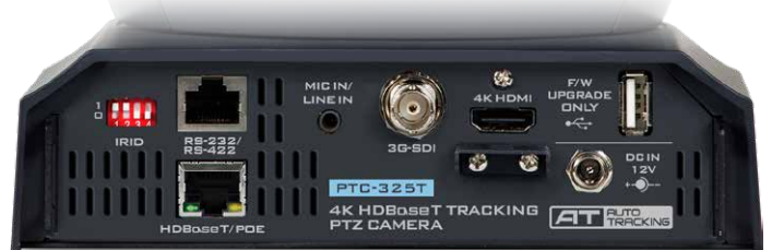
PTC-325T Rear (HDBaseT Output)
